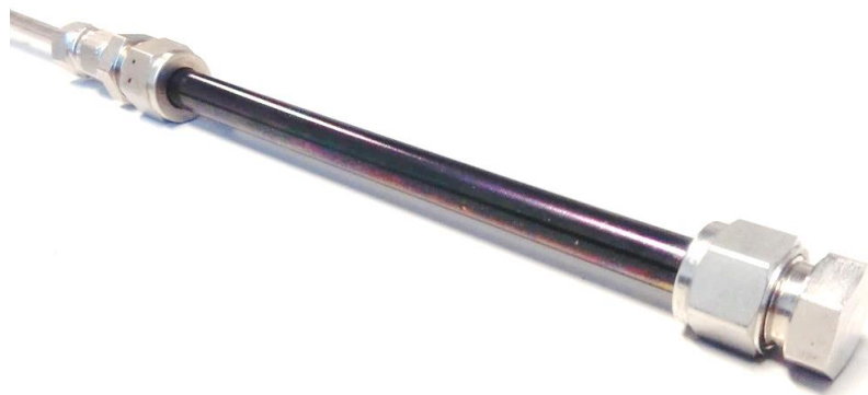
Figure 5.1. A Pd-Ag double-skinned membrane (150 mm long) with a ceramic protective layer supported onto an \alpha\text{-Al}_2\text{O}_3 porous support and sealed with graphite-based seals.
