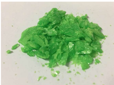
Figure 6.5. The green ferrioxalate crystals as obtained after synthesis and three times recrystallization.
