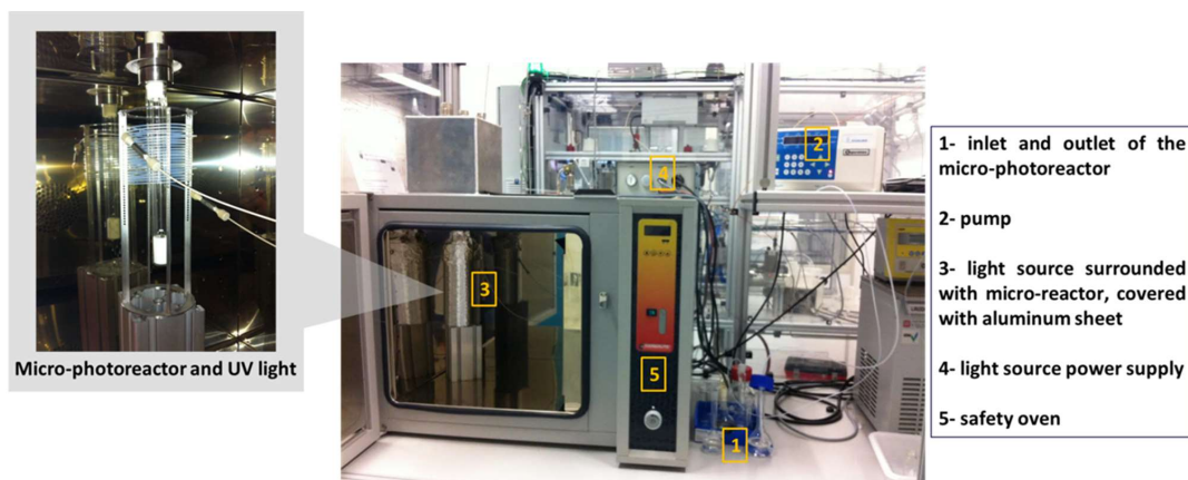
Figure 8.1. Micro-flow setup for photoisomerization and in-flow separation process
