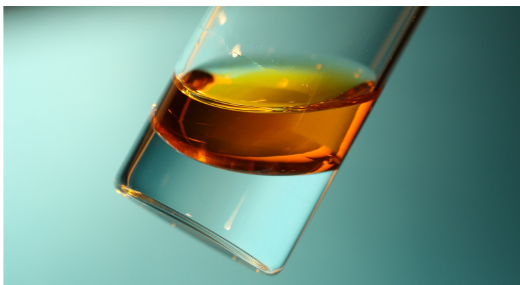
Figure 2.2: DecA: N_{8888}-Br (2:1) after mixing with water. A 1:1 mass ratio of DES and water was used.
