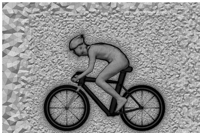
Fig. 26. Computational grid in vertical center plane. Cell count: 55.3 million.
