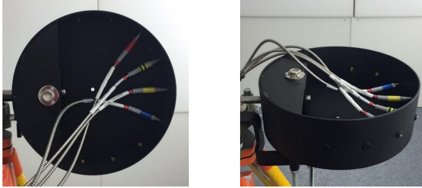
Figure 4. The multidirectional spectroradiometer ( MuS ) in vertical (above-left) and horizontal (above-right) position, as well as the configuration of the fibers in vertical (below-left) and horizontal (below-right) positions.
