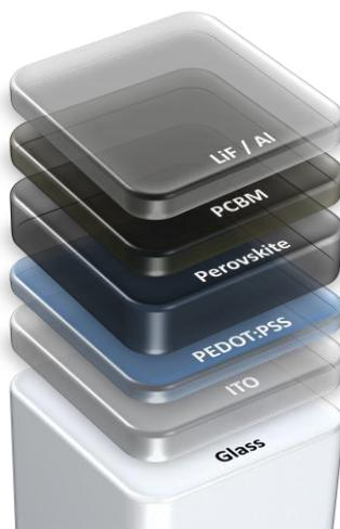
**Figure 3.1** The solar cell stack that is used for the optimization of the perovskite layer for high solar cell efficiency as described in this chapter.
