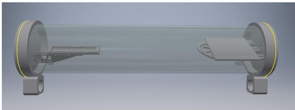
**Figure 5.6** Schematic representation of the designed VASP reactor with the temperature controlled sample stage on the right and the crucible on the left inside a Pyrex tube with stainless steel end caps. It must be noted here that the crucible shown here was changed for a much smaller ceramic piece.
