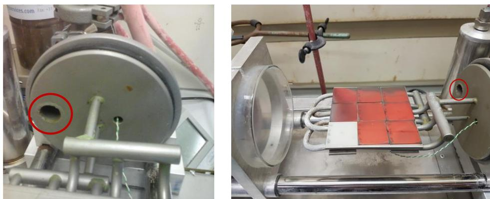
**Figure 5.12** Pictures showing the position of the chambers' exhaust (red circle) with respect to the sample stage.
