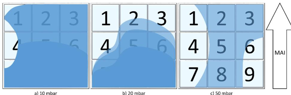
**Figure 5.11** Influence of chamber pressure as regulated by introducing N<sub>2</sub> gas on the obtained deposition profile where a darker color equals a thicker MAI layer.
