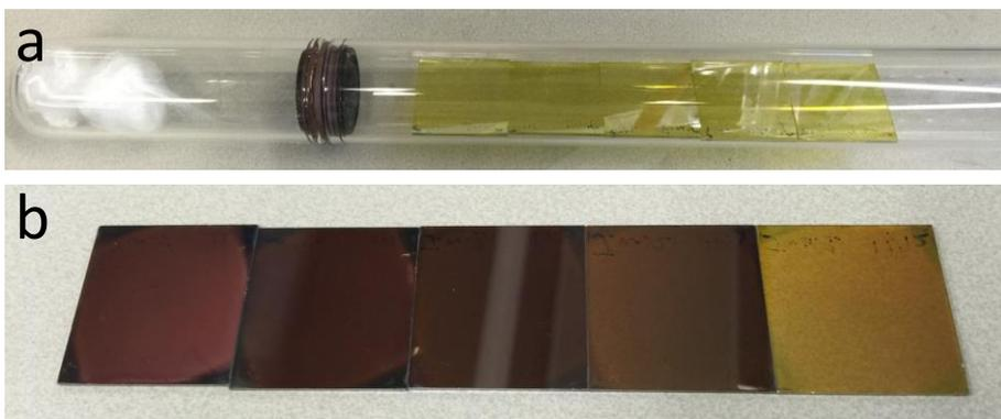
**Figure 5.5** Example of the MAI crystals covered by wadding and porous  $\text{PbI}_2$  (120  $\mu\text{l TBP mL}^{-1}$  DMF) covered substrates inside the glass tube before deposition (a) and the finished layers after the complete 100 min. deposition process (b).
