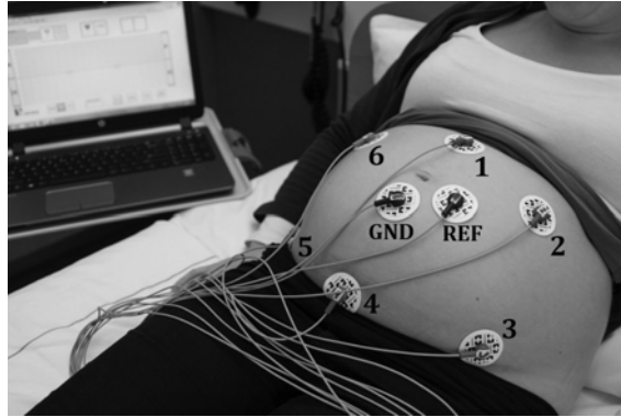
Figure 8.2: The six channel fetal electrocardiogram is recorded with electrodes on the maternal abdomen, placed in a fixed configuration. The ground (GND) and reference (REF) electrode are placed near the belly button. The electrodes are connected to a battery operated data acquisition system (Nemo Healthcare BV), which filters, amplifies, and digitises the data for further processing. This system is connected to a computer.
