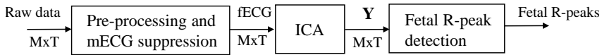
Figure 4.1: Block diagram of fetal heart rate detection. M is the number of channels and T is the total time of the recording.
