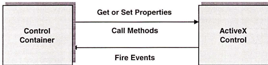
Figure 10 control container communication
