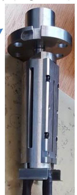
Figure 5: Custom-designed piece to visualize flow front
