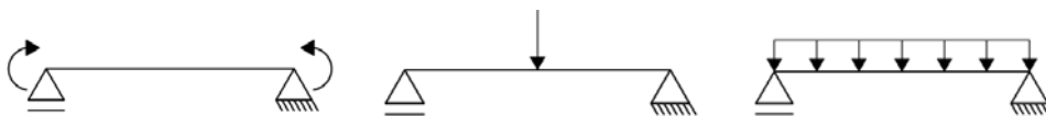
Fig. 1: Three load cases (LC) considered: LC1 – constant bending moment (left), LC2 – concentrated load (middle), LC3 – uniformly
