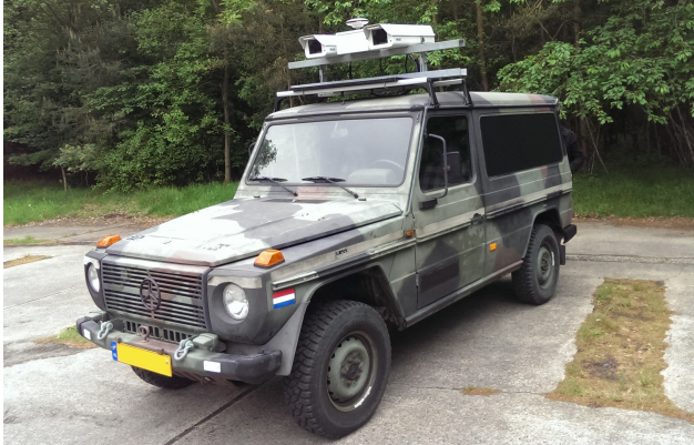
Figure 3: Prototype vehicle used for our experiments, featuring a stereocamera with 1920 \times 1440 pixel resolution and GPS/IMU positioning, achieving decimeter accuracy.
