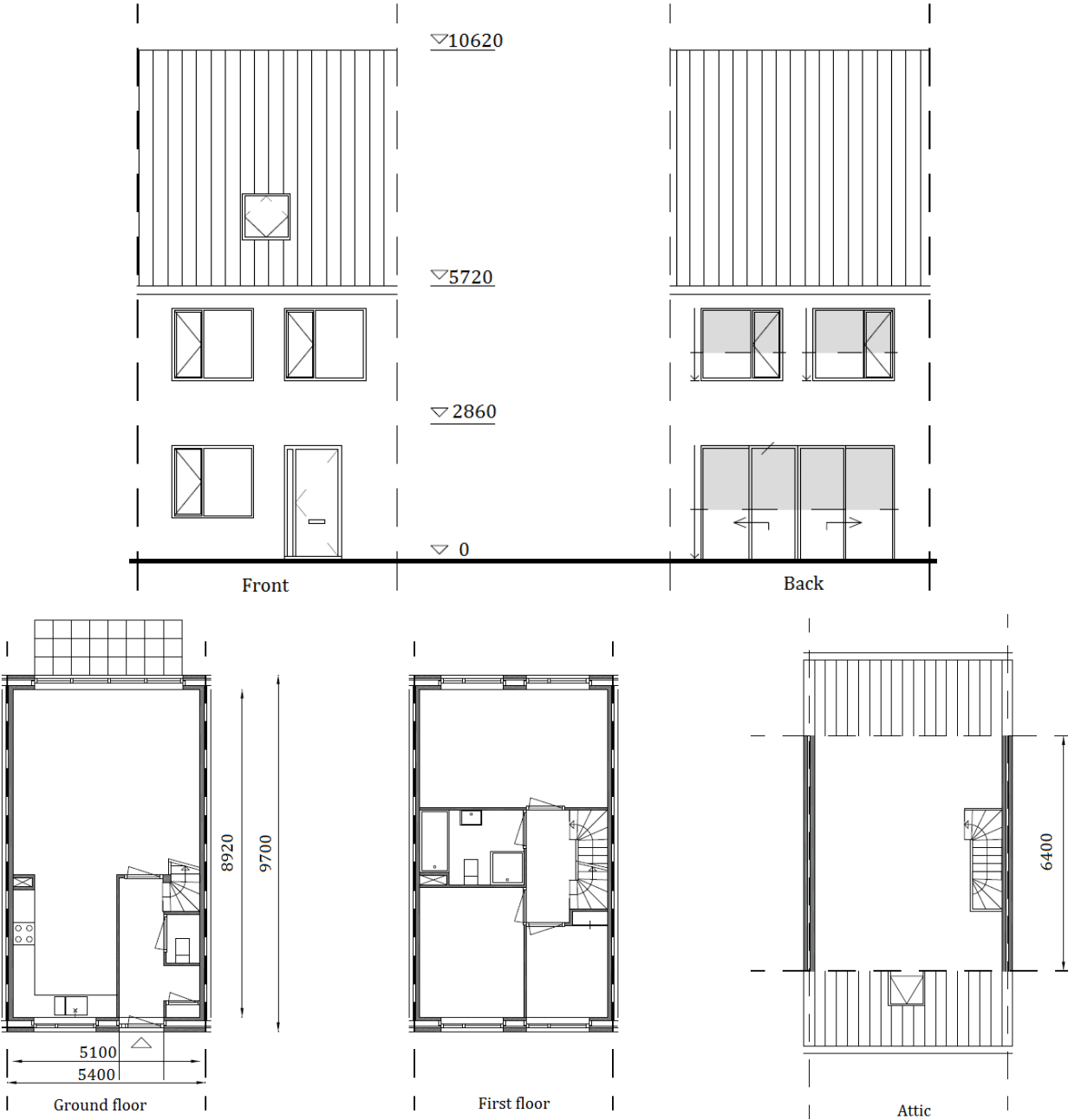
Figure a Layout of a typical Dutch terraced house, showing different floors, front and back view of the building. All dimensions are in mm.
