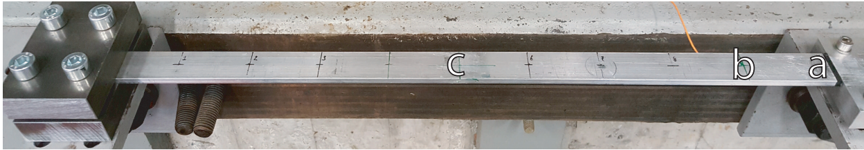
Figure 8: Experimental clamped-free aluminum beam set up.
