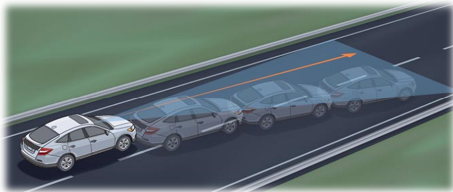
Figure 2: Lane Centering System [24]
