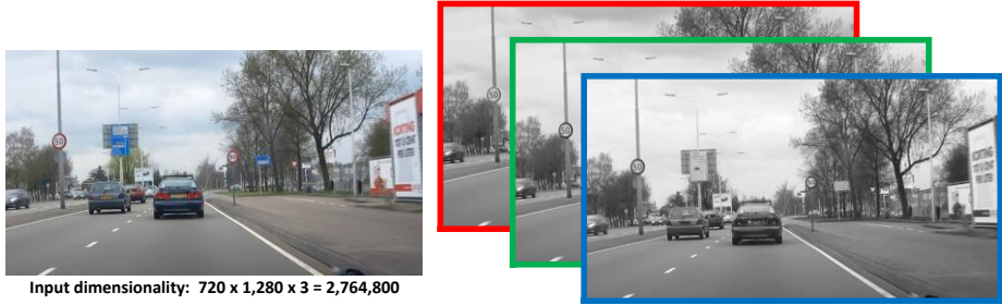
Figure 2.1: A 720 x 1,280 RGB road scene image for speed sign recognition has a huge input dimensionality of 2.76 Million input variables.
