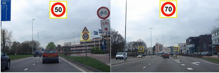
Figure 3.1: Speed sign detection and recognition by an in car camera. Speed signs occur on different locations and with various scales depending on their distance.
