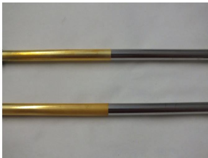
Figure 1. Picture of two membranes (half Pd-Ag and half Pd-Ag-Au) prepared by ELP (picture taken before annealing treatment).
