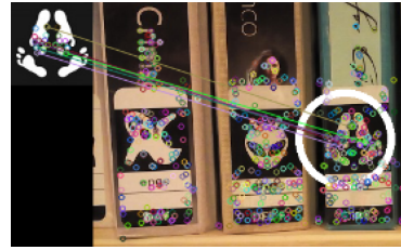
Figure 8. Example alternative technology tested in BLIIPS: processing the visual appearance of book spines to recognize pictograms denoting book types.
