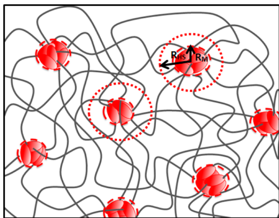
Figure 4. Physically cross-linked network of PEG-DFA hydrogels; DFA hydrophobic aggregates (in red) and PEG chains (in black). R_{HS} is equivalent hard sphere radius according to Percus–Yevick model; R_M is mean micellar radius.
