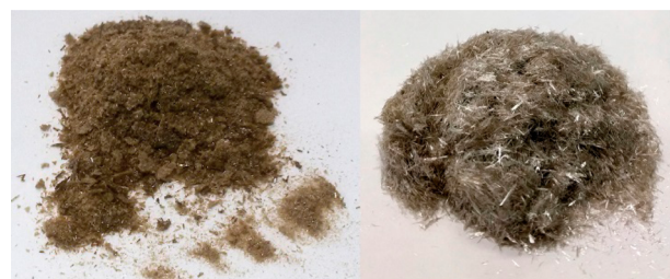
Figure 2. Comparison of the solids obtained after precipitation of di- p -tolyliodonium triflate ( 3a ) produced either in batch (left) or flow (right).
