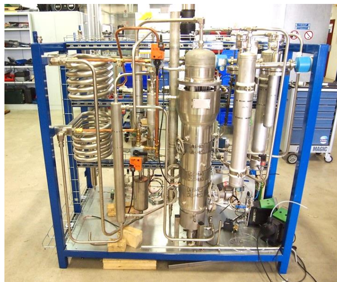
Figure 16. Skid with fuel processor.
