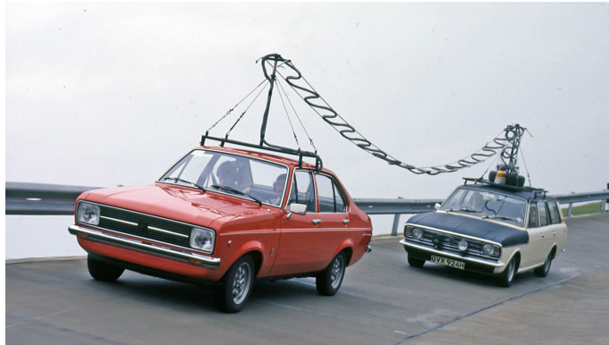
Figure 1.3. Communicating cars, not long ago communication between cars was a dream. The use of ‘tethering’ permitted bulky recording equipment to follow in the vehicle behind without affecting the test vehicle. Source: Ford of Britain 100: Image of the week - 18/52 © [2011] Ford.co.uk
