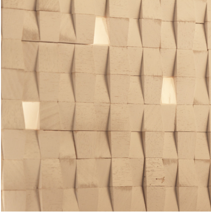
Wall of 1:20 model made with BinAir building system
