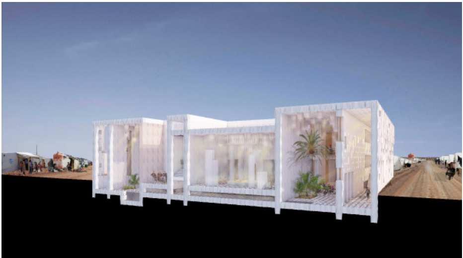
3D section through buffer zones, central axes and hot room
