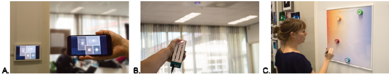
Figure 1. Photos of the interfaces: (A) the Floorplan interface displays a map of the space where light can be adjusted; (B) the Pointer as remote control for the light; and (C) the Canvas interface with tokens that can be moved around to change the light.
