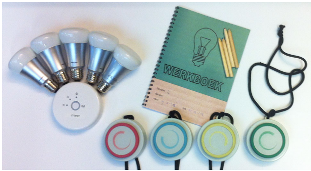
Fig. 3 Probe set, consisting of Philips Hue bulbs, mobile dimmer controllers, and a workbook
