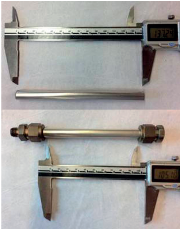
Figure 3.4 Pd membrane (E80 – Pd-Ag membrane, thickness 4.5 micron) before and after connecting to the Swagelok® connectors.
