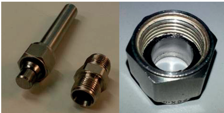
Figure 3.3 Left: 316L dummy rod with graphite ferrule and Right: connector with pre-treated ferrule (shiny inner surface)
