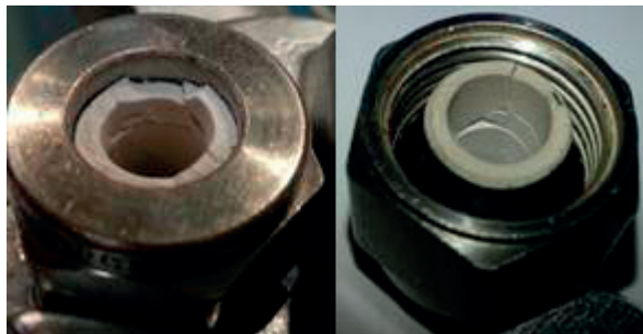
Figure 3.5 Broken Membrane after applying 14 N.m.
