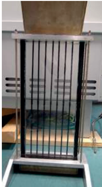
Figure 6.4 Front view of the glass column with immersed vertical tubes and spacers (distance between the membranes: 31 mm, distance from the reactor wall for the most right and left membranes: 32 mm)
