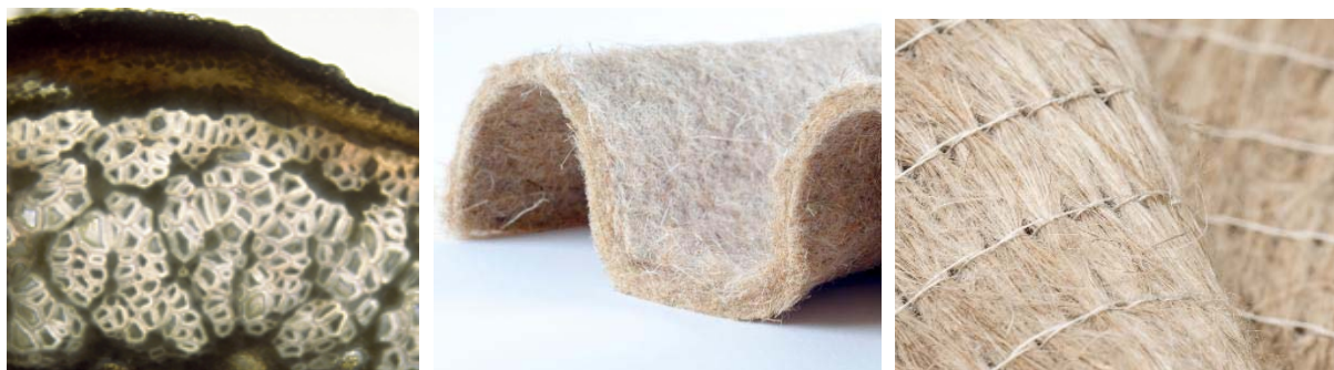
Fig. 1: Cross-section of hemp fibres under the microscope
