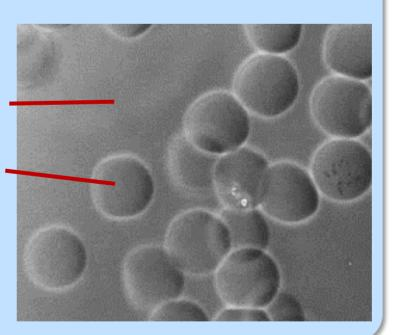
The beads are embedded in a collagen I hydrogel without loss of material or mixing, as shown by a CNA35-OG probe for collagen.
