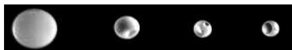
FIG. 9. Shell formation around an evaporating droplet, resulting in highly asymmetric phosphorescence intensity profiles.
