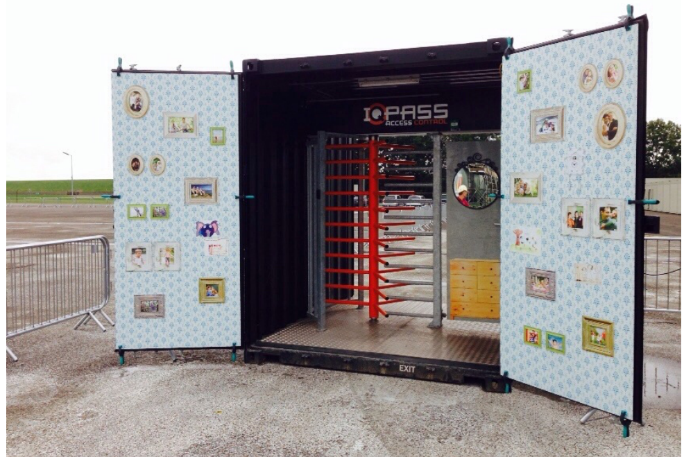
Figure 2 – Transition gate into the 'unsafe' workspace
