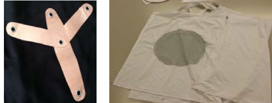
Figure 2. (a) The PCB shape in a Kapton polyimide film, attached to fabric using Anorak snaps. (b) Double layer with mesh fabric to adjust the PCB in the Wrap top.
