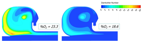
Figure 3 – Damköhler number contours in the mid-plane of the combustor for two different oxidizer compositions. Simulations including radiation modelling.
