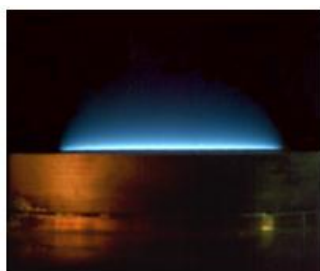
Figure 1: A flat plate/heat flux burner (left) and schematic section view of the new burner head (right).
