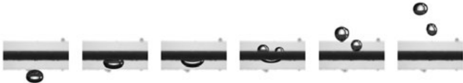
Figure 7.2: Image sequence of a bubble which has its centroid aligned with the wire rib. The time interval between the images is 0.12 s.
