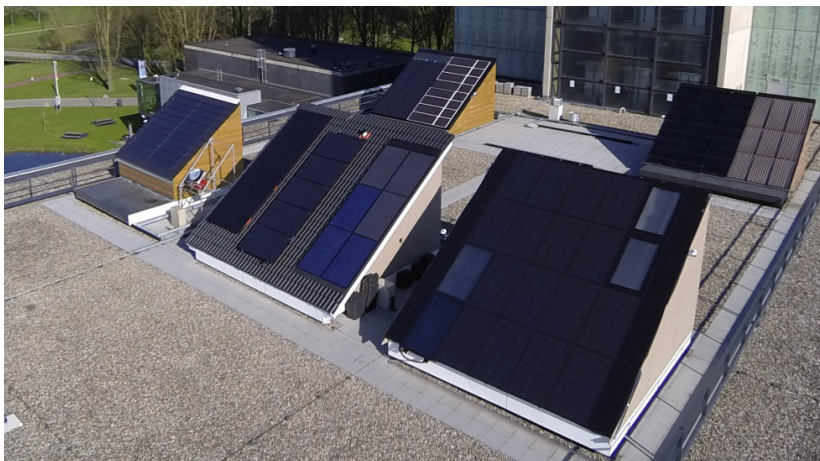
Fig. 1. Field test facility Solar BEAT. The middle dummy building in the front row contains the three types of uncovered PVT systems.
