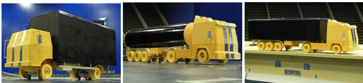
Figure 1: Scale vehicle models: VAN (left), tanker (centre), truck (right).
