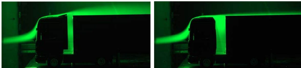
Figure 10: Smoke visualization with and with no installed roof and side extenders.
