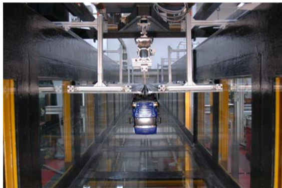
Figure 23: Installed truck model in WSG.
