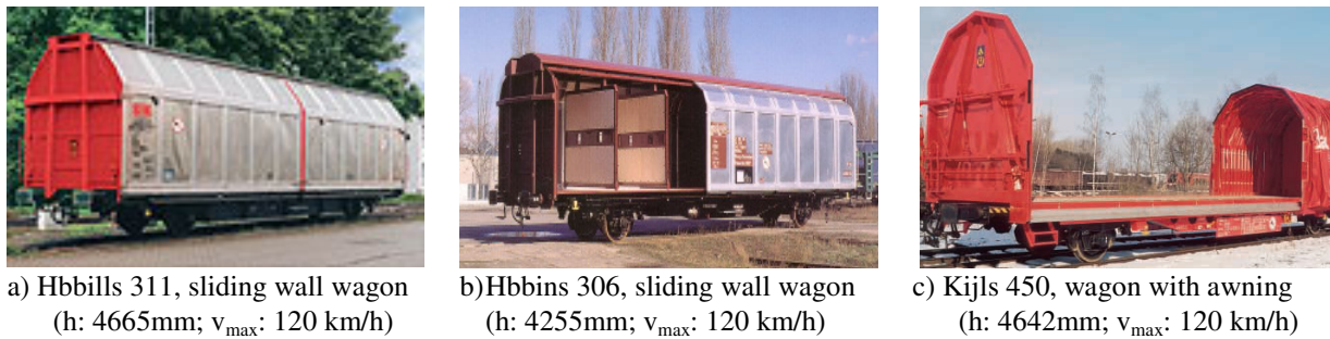
Figure 1: Three examples of freight wagons investigated with respect to cross wind stability.
