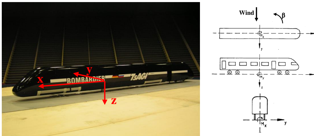
Figure 5: Aerodynamic coefficients' sign convention
