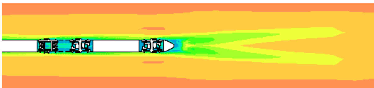
Figure 6: Velocity magnitude at the rear side of the train
