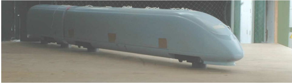
Figure 2: ICE 3 model on an elevated splitter plate in the test section of the GroWiKa
