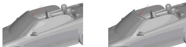
Figure 15: Spoiler on the wind shield (left) and unattached spoiler (right).
