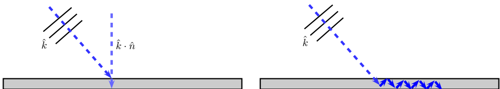
Figure 1.3: Locally reacting and non locally reacting liners respectively.
