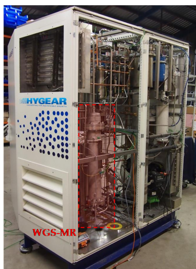
Figure 13. Picture of the prototype reactor for WGS process where the placement of the WGS-MR is highlighted.
