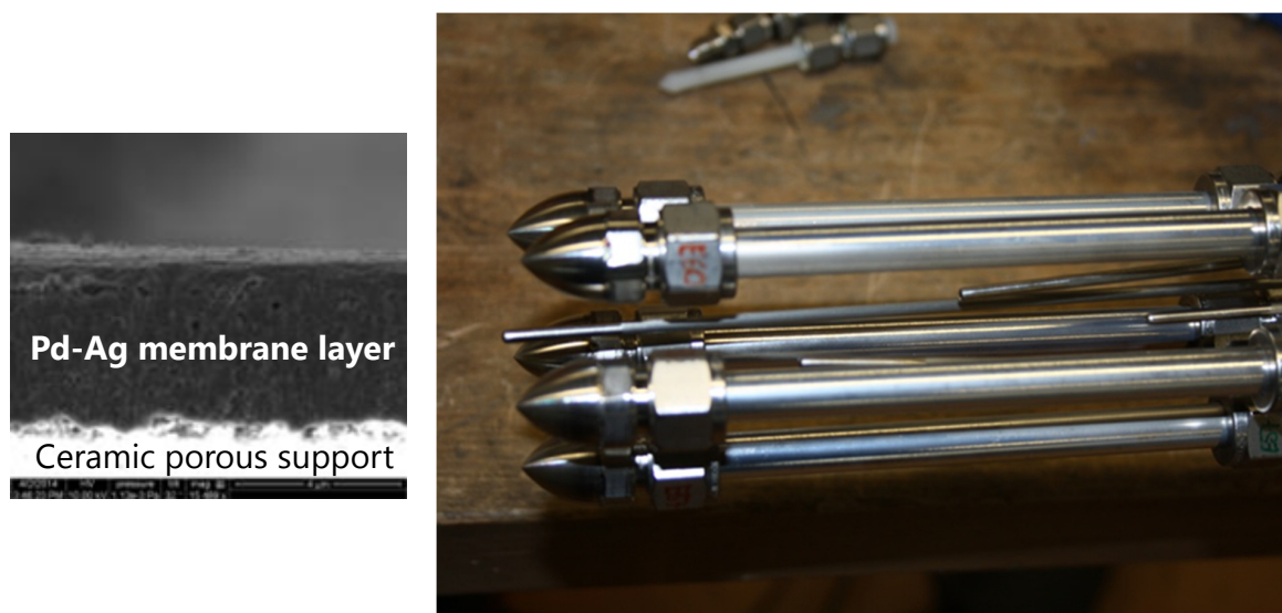
Figure 6. (Left) Cross section of a Pd-Ag membrane; (Right) Pd-Ag membranes to be integrated in the lab-scale reactor.
