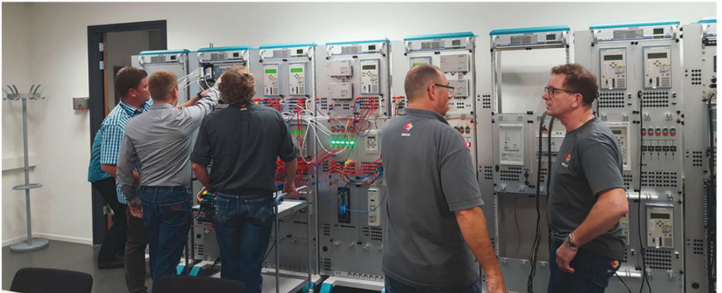
A new hardware training simulator is in use at the new training center for protection, automation and control equipment.
