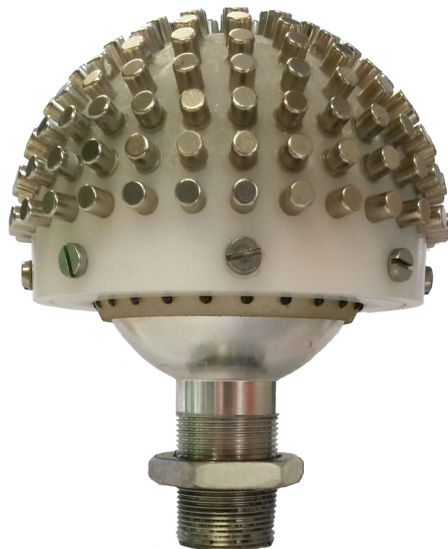
Figure 6.3: Photo of the spherical gravity compensator prototype.
