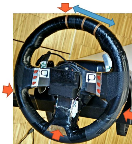
Figure 10. The six gestures for the embedded WheelSense system based on capacitive sensors: hand tap in the top/bottom/right side/left side, and hand swipe up/down.
