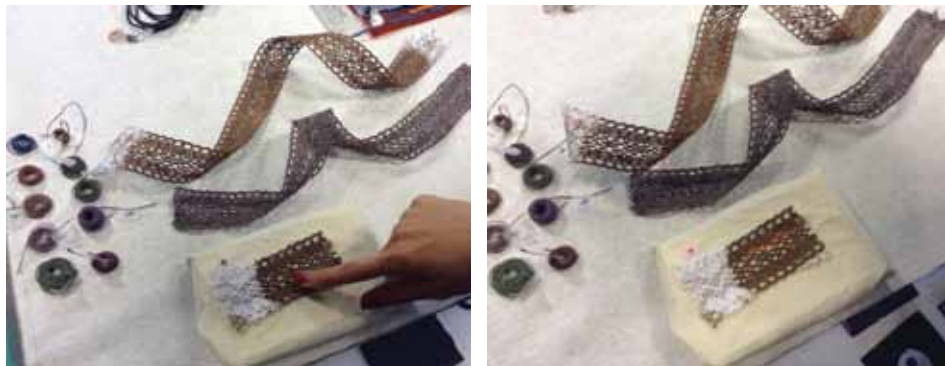
Figure 38 Butterfly lace, that heats up an integrated conductive yarn when touched. The temperature change causes the yarn in the thermosensitive lace to change colour.
