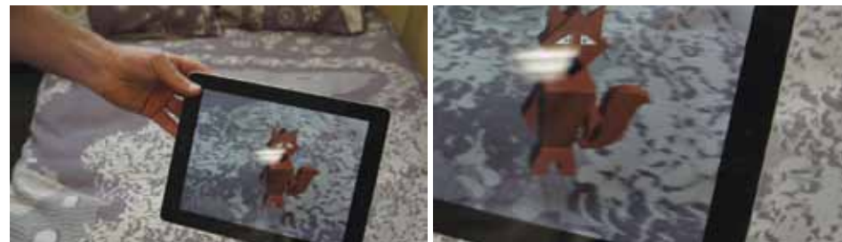
Figure 48 The camera of the iPad has recognised the marker on the Bedtime Stories duvet cover, and the application projects the 3D character in the Augmented Reality layer.
