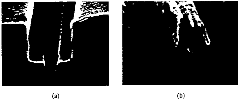
Figure 2.8 (a) Two-level resist profile after e-beam definition and development; (b) Resulting gate metal profile with a footprint of 0.15 \mu\text{m} and a top of 0.7 \mu\text{m} .
