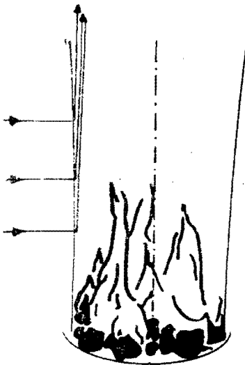
Fig. 2.2. Stream lines of entrained air
