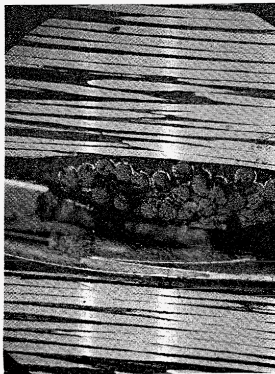
FIGURE 35: A tested dry woven nylon substrate with a nickel layer (enlargement is 315).
