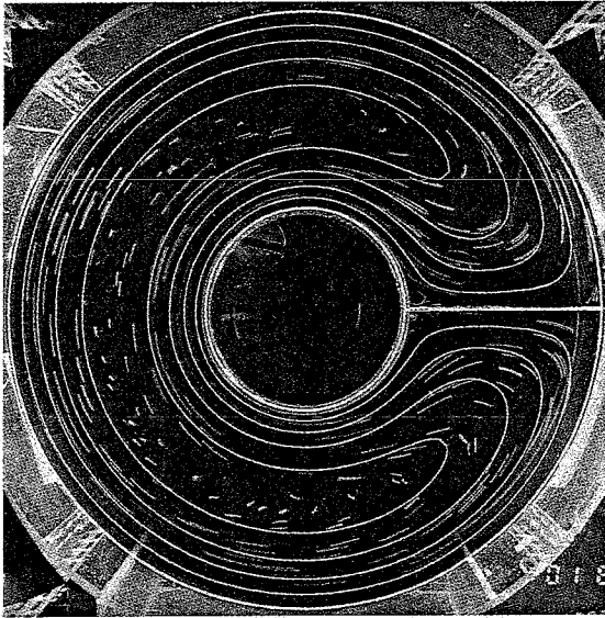
Figure 1: The starting flow in an annular tank with a radial barrier.
