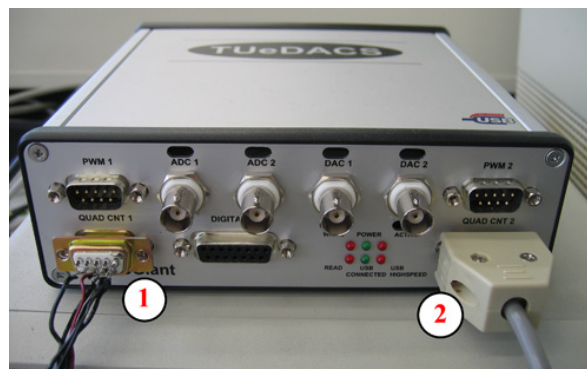
1. Quadrature input low res enc 2. Quadrature input high res enc
