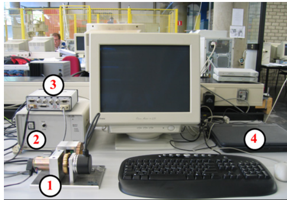
1. Mechanical system 2. Amplifier 3. MicroGiant 4. Notebook
