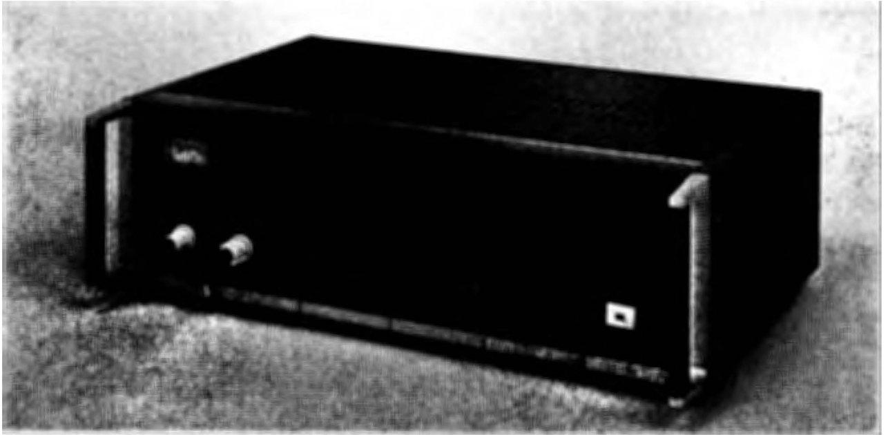
Fig. 13. The DAMA annoyance meter ('Drop-out Annoyance Measuring Apparatus'), which automatically determines the annoyance ratings of drop-outs in the signal on an audio tape.
