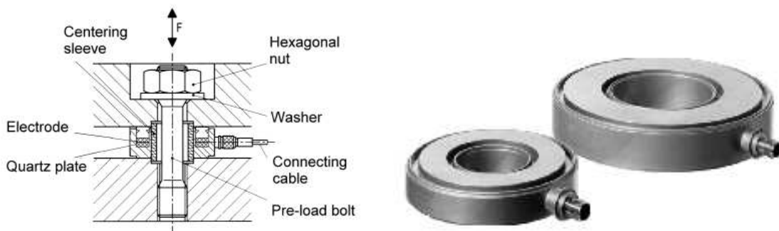
Figure 4.4: Design of the piezo sensor (left) and mounting of the sensor (right).
