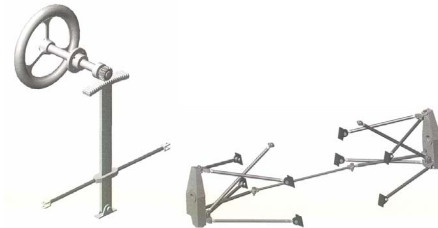
figure 7: a) steering wheel b) steering system with tie rods
