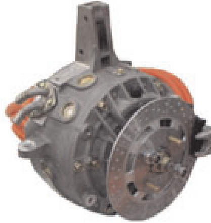
Figure 3.5: Mitsubishi's MIEV in-wheel motor design
