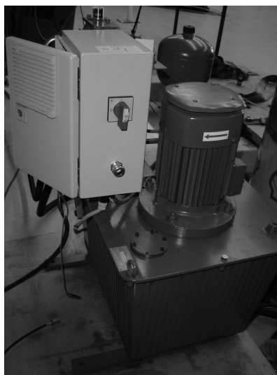
Figure 2.4: hydraulic power unit [Rexroth-Hydraudyne]
